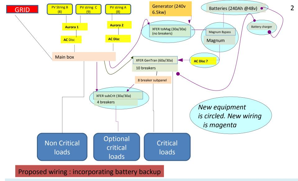
This setup maintains the current wiring, and treats the battery backup (Magnum + batteries) as the generator. A generator that is preferred to the grid!
