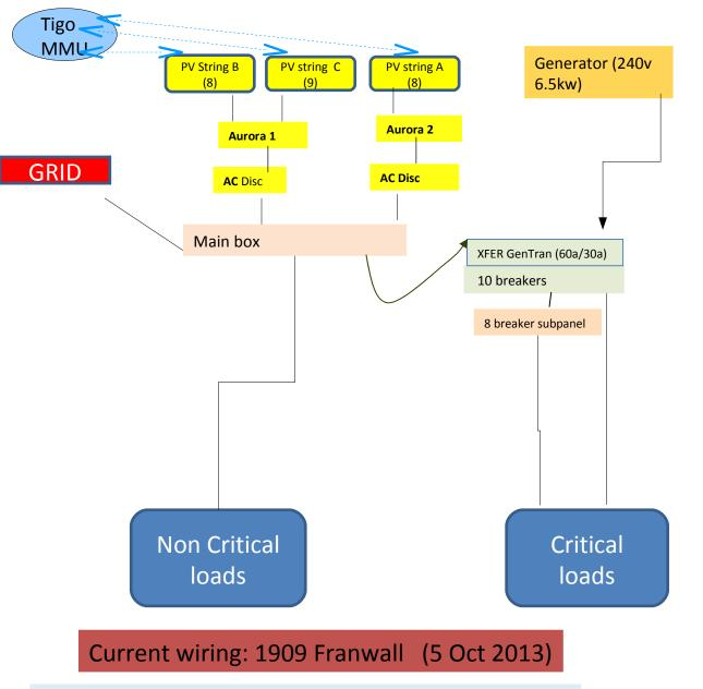
The 8 breaker subpanel is, functionally, part of the XFER\_GenTran. It was added to meet code requirements for dual breakers on multi-branch lines.
